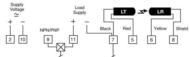
Transistor output – PA 10 A/B 61X
