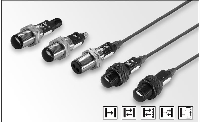
The 7000 series consists of a self-contained transmitter SMT, and a receiver SMR which are to be used in thru-beam mode, an SMP for diffuse proximity, SMRR for retro reflective and an SMPF for use with fibre optic cables. All are offered with sensitivity adjustment via integral potentiometer with either cable or plug connection.
