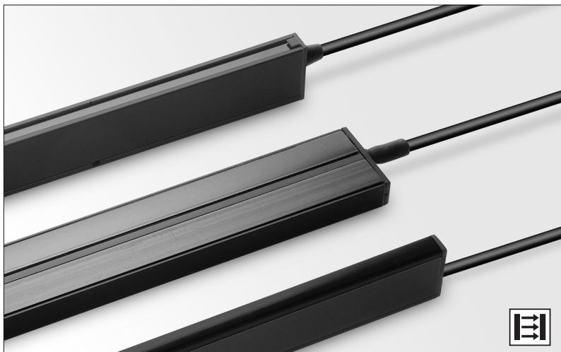
The SG 1 light curtain system consists of a self-contained transmitter detector, SGT and receiver detector, SGR, which are to be positioned opposite of each other. The detectors are housed in a sturdy aluminium profile available in a slim line design (10 x 28 mm), a leading edge design (37,5 x 13 mm) and a water-resistant slim line design (12 x 30 mm).
