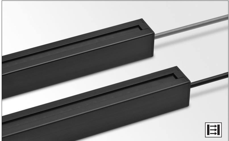
The SS 01 series is a light curtain system which consists of a self-contained transmitter SST and receiver SSR, which are to be positioned opposite of each other. The detectors are housed in a sturdy aluminium profile (33 x 36 mm) with T-slot mounting rail, available in lengths ranging from 160 mm to 1980 mm.
